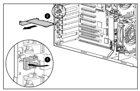
Figure 2-30. Removing a Netelligent 10/100 TX UTP PCI Controller
